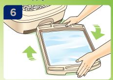
Slide drawer out to replace the disposable pad weekly. Drawer can also be rotated without touching the pad, to distribute liquid evenly across the pad.
